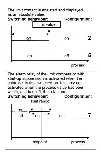
on: Relay "activated" off: Relay "not active"
