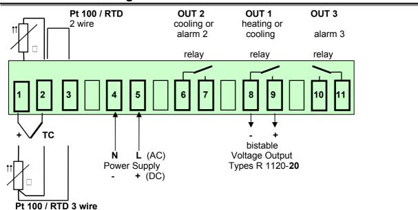
It is not permitted to connect the grounds of the sensor- and bistable voltage outputs with each other.
